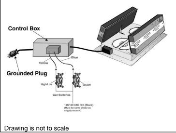
The HV whole house cooling fans are not for use with solid state speed controls
